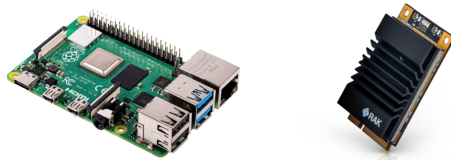
Figura 15: Raspberry Pi 4B + RAK2287.
